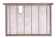
4) It is also useful a 2cm thickness and  $5.5 \times 9$ cm dimension plank, that is to be laid over the foundation in order to cut a rectangle.
